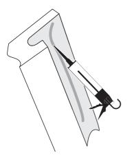
Once inserted, flatten the panel against the wall and smooth any excess adhesive across the joint to cover any missed areas.
