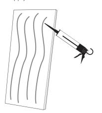
Before applying TopSeal, clean the edges or tongues and grooves to remove any dust that may interfere with the sealing process. Ensure that when joining two panels, the surface is flat to avoid any issues during the installation process.
