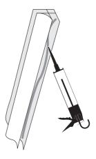
When butt jointing two flat-edged panels, apply a thin bead of TopSeal to one panel, distributing it evenly.
